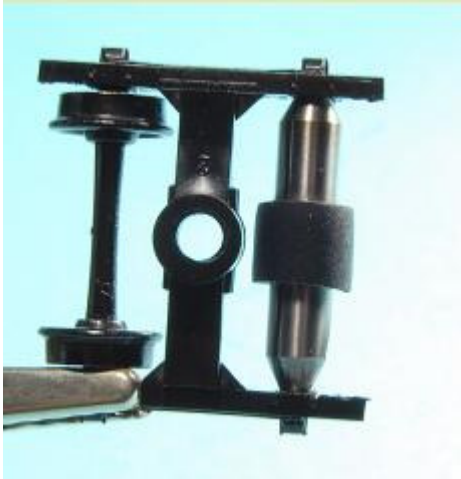
A "Reboxx HO T-100 Exxact Socket Tool" is used to open up the sideframes to accept the longer axles.
