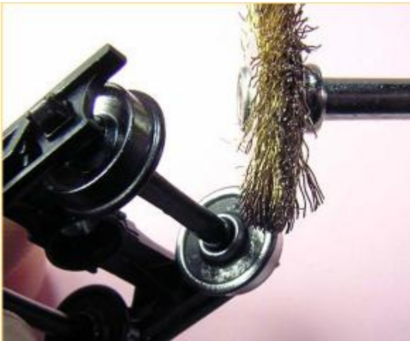
The Kadee wheelsets have a coating that doesn't conduct electricity. Put the wheelset in an EXPENDABLE truck frame and burnish the wheels with a brass brush in a motor tool.
