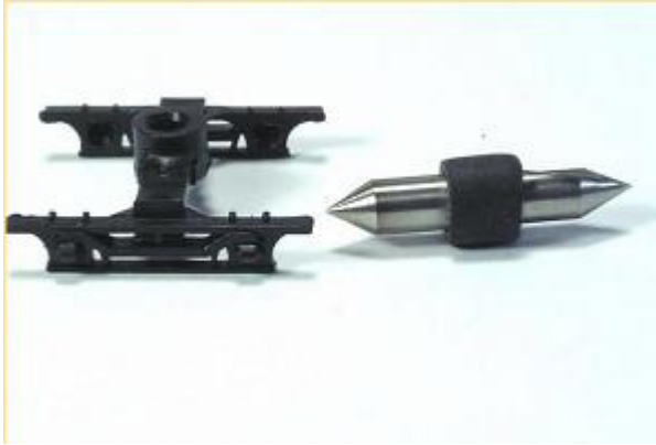
A "Reboxx HO T-100 Exxact Socket Tool" is used to open up the sideframes to accept the longer axles.
